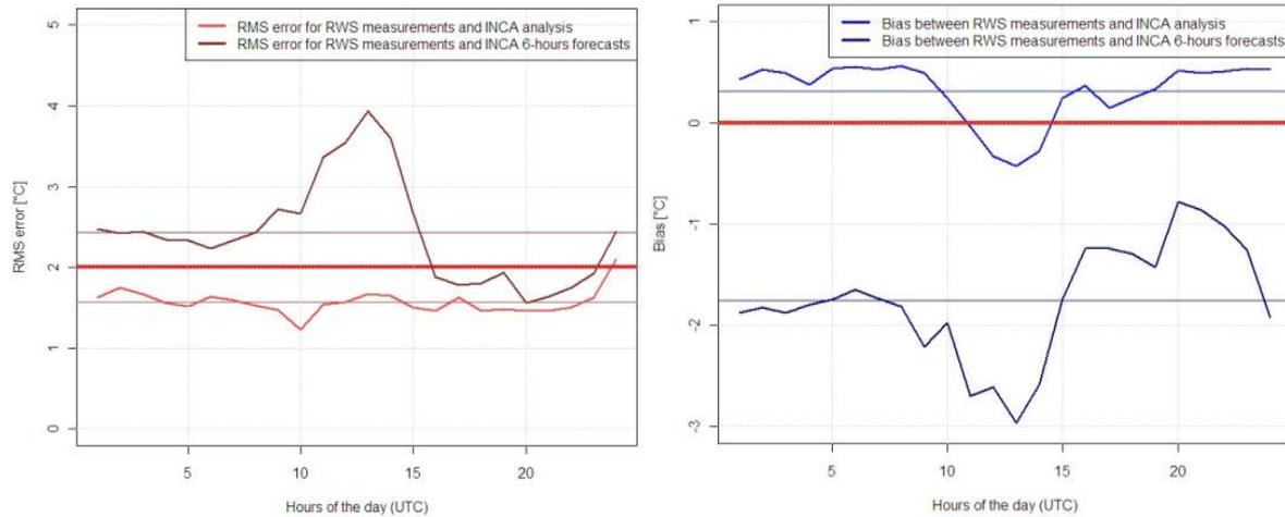
Figure 3. RMS error (left) and bias (right) for RWS *Jeprca*, calculated for each hour of the day between INCA surface temperature analysis and 6-hour forecasts, and RWS RST measurements. Average RMS error and bias are denoted with thin horizontal line and 2°C / 0°C line is denoted with heavy horizontal line.
