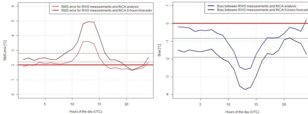
Figure 4. RMS error (left) and bias (right) for RWS *Mislinja*, calculated for each hour of the day between INCA surface temperature analysis and 6-hour forecasts, and RWS RST measurements. Average RMS error and bias are denoted with thin horizontal line and 2°C / 0°C line is denoted with heavy horizontal line.
