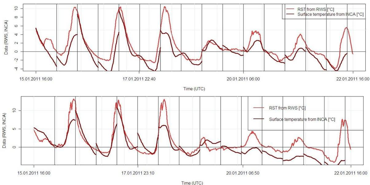
Figure 2. INCA surface temperature forecasts (from 0 to 11 hours ahead) compared by RST measurements from RWS *Jeprca* (top) and RWS *Mislinja* (bottom) for the selected time period. Dark vertical lines denote INCA forecast starting point (analysis).
