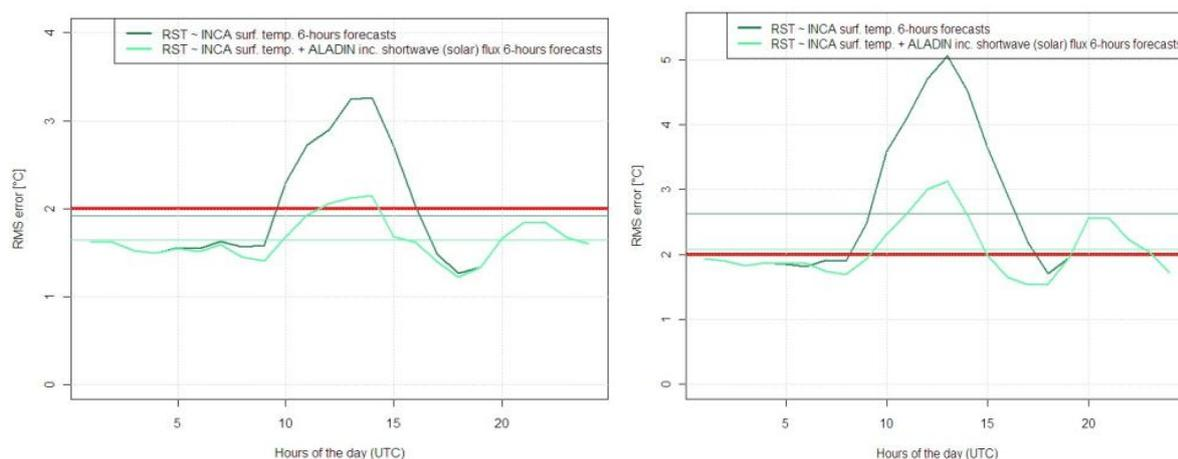
Figure 8. RMS error for regression equations (1) and (2) at RWS *Jeprca* (left) and RWS *Mislinja* (right). Average RMS error is denoted with thin horizontal line and 2°C line is denoted with heavy horizontal line.
