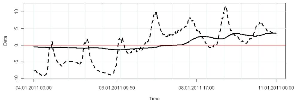
**Figure 3:** Road surface (dashed line) and subsurface (solid line) temperature measurements on RWS *Mislinja* from 4 to 11 January 2011.
