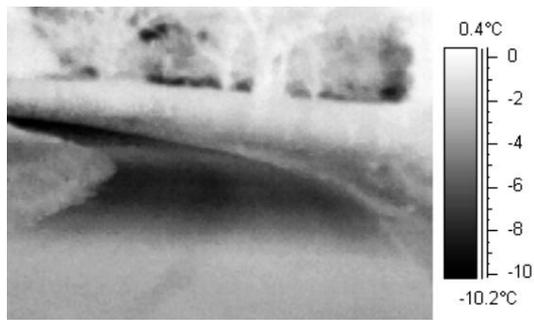
**Figure 1:** Thermal image of road showing a great variation of RST in relation to the shading from trees [15].
